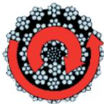
The geometrical design of rotation-resistant CASAR Special Wire Rope is such that the moments in the core and the outer strands compensate each other over a wide load spectrum, so that even with great lifting heights no rope twist occurs.
